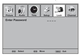
3 Press the number buttons to enter the four-digit password. The default password is 0000. The Lock menu opens.
